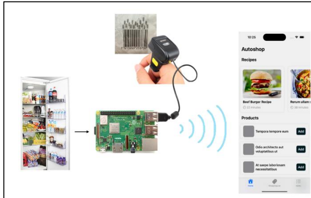
Figure 1. Working principle of the developed smart refrigerator
